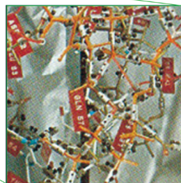
FIGURE 9. As seen in Figs. 2 & 3, the first protein structures were physical models built from brass components, known as Kendrew Models. In 1968, together with Yuval Eshdat, I built this model of hen egg white lysozyme using coordinates determined by David Phillips (Fig. 4) and sent on a computer printout to Nathan Sharon, Yuval's PhD supervisor. Such manual modeling was slow and difficult but it provided me the impetus to do the first energy calculations on an entire protein (Fig. 10).
